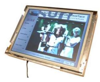
15" Screen Multi-Media Kiosk Panel PC with Fanless 1 GHz VIA Industrial M/Board, 256 Mb RAM, 40 Gb HDD and Windows O/S
